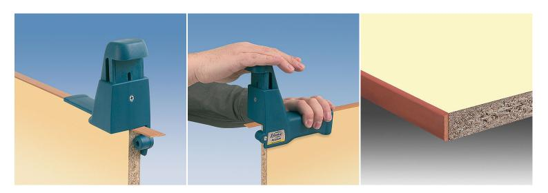
Manual end trimmer for PVC, melamine, polyester, veneer, etc... up to a maximum thickness of 2mm. The maximum width to cut edge bands is 45mm. The trimmer makes a perfect, clean cut at all corners of the board. Equipped with sharpenable blades and a special system to adjust the cutting position.
