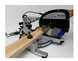
The TT255SL is a mitre saw with pull function and the little sister of the TT305SLX. It is equipped with a noiseless 1600 W induction motor that requires no maintenance (which is a big advantage over the carbon brush motor in the smaller models) and has a pull function up to 300 mm, with a cutting height up to 60 mm.
