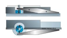
Use the adjustment ruler to always correctly set the depth and height of your milling or saw cut in relation to your guide. Scale per mm.
