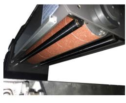
This compact and professional open-end drum sander with variable speed control offers you tremendous versatility and large sanding capacity for any small work area. Thanks to the open stable base, a sanding width of up to 915 mm and a sanding thickness of up to 127 mm is possible.
