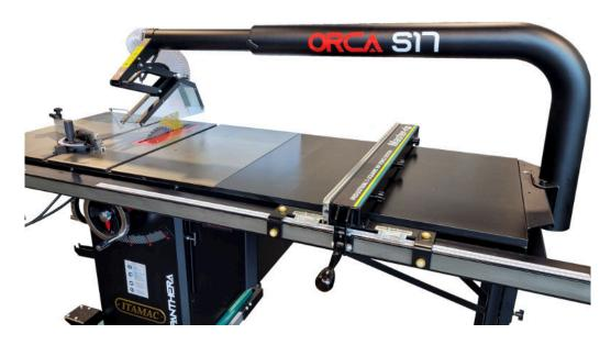
The saw table insert is designed for use at any cutting angle and can be easily removed thanks to the **magnetic attachment** in the table. Through fine adjustment, this plate can also be adjusted for a 100% flat transition with the cast-iron table top.
