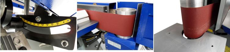
The TT2600 KSM has a very stable and strong machine frame that eliminates vibration. The sanding unit can be tilted to 45 degrees. The height of the work surface is adjustable (185 mm) so that the 2600 x 150 mm sanding belt is fully utilized. The machine is equipped with a contour table for sanding curves. The tension rollers are equipped with springs to compensate for the stretching of the sanding belt. The sanding belt has grit 100 as a standard, but is also available with grit 60, 80 and 150.
