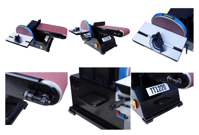
The sander TT1220 can be used vertically, horizontally or at any angle. The large aluminium table can be tilted up to 45° and is equipped with a protractor. The work table is supported on both sides for precision use. It features a D handle for easy transport, and a quick-release sanding belt system for quick changes. The belt can be easily balanced thanks to the handy control knob. The machine also has a 60 mm extraction outlet.
