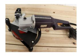
This powerful diamond wall cutter is designed for pulling trenches for power lines. The device is equipped with high-quality electronics with built-in overload protection. At the same time, a current limitation was provided when the device was started up. This enhances safe and correct use, even for beginners. The desired milling width can be set quickly. Finally, it is possible to connect a hoover directly to the unit, which makes work considerably easier.
