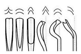
Ideal for regrinding curved tools, gouges, cutting and woodturning tools. Convex and concave diamond surface in one grinding tool. Re-grinding of tools with a radius of min. 1.6 to max. 25 mm. Includes non-slip pad for easier use. No oil required - grind dry or with water.
