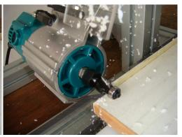
With this edge router, you have affordable automation. Large adjustable carrier plate covered with Teflon carriers. You mill the side, corner and top in one movement from right to left.
