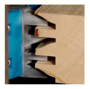
Set of profile knives of height 40mm Nr. 0026 suited for universal moulding blocks. Used for moulding of wood at low costs. The steel alloy with 16% cobalt guarantees a high quality cut and a comfortable cutting process.
