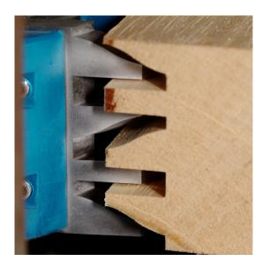
Set of profile knives of height 40mm Nr. 0027 suited for universal moulding blocks. Used for moulding of wood at low costs. The steel alloy with 16% cobalt guarantees a high quality cut and a comfortable cutting process.
