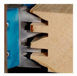
Set of profile knives of height 40mm Nr. 0031 suited for universal moulding blocks. Used for moulding of wood at low costs. The steel alloy with 16% cobalt guarantees a high quality cut and a comfortable cutting process.
