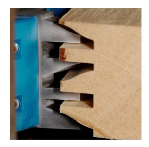
Set of profile knives of height 40mm Nr. 0047 suited for universal moulding blocks. Used for moulding of wood at low costs. The steel alloy with 16% cobalt guarantees a high quality cut and a comfortable cutting process.
