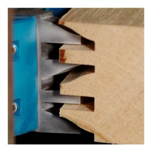
Set of profile knives of height 40mm Nr. 0089 suited for universal moulding blocks. Used for moulding of wood at low costs. The steel alloy with 16% cobalt guarantees a high quality cut and a comfortable cutting process.
