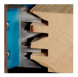
Set of profile knives of height 90mm Nr. 5302 suited for universal moulding blocks. Used for moulding of wood at low costs. The steel alloy with 16% cobalt guarantees a high quality cut and a comfortable cutting process.
