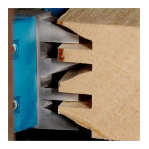
Set of profile knives of height 90mm Nr. 5326 suited for universal moulding blocks. Used for moulding of wood at low costs. The steel alloy with 16% cobalt guarantees a high quality cut and a comfortable cutting process.
