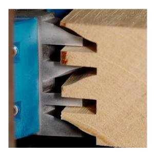
Set of profile knives of height 90mm Nr. 5330 suited for universal moulding blocks. Used for moulding of wood at low costs. The steel alloy with 16% cobalt guarantees a high quality cut and a comfortable cutting process.
