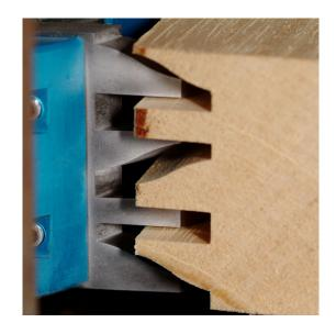
Set of profile knives of height 90mm Nr. 5351 suited for universal moulding blocks. Used for moulding of wood at low costs. The steel alloy with 16% cobalt guarantees a high quality cut and a comfortable cutting process.
