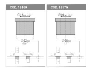
These adapters are made for the TCP piston clamp and ensure that it can also be used on welding tables with a
