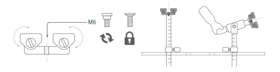
This tube adapter is made for the TCP Piston clamp. Galvanized and made of carbon steel. Accessory can be fixed or rotatable depending on the chosen screw.
