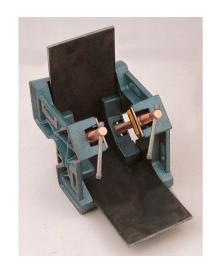
Strong angle clamps for welders. Mounting at 90  $^{\circ}$  is no longer a problem. The pressure height is 3.5cm or 6cm and can clamp material up to 8.5cm or 12cm width. Made of nodular cast iron and equipped with copper-plated
