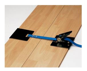
This band clamp is specially designed for installing parquet. The band clamp has a length of 5 meters and is equipped with two metal corner plates so that you can easily pull parquet and laminate together. Pressure up to 800 kg.
