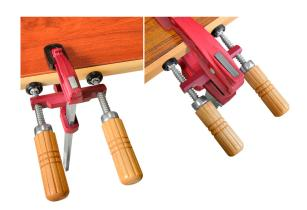
This double edge clamp can be used on all types of glue clamps with a thickness of maximum 10mm thickness. It is made from a steel body and has a galvanized thread. The handle is ergonomic and made of beech wood. Includes plastic protective cap. The edge clamp can be rotated out by a maximum of 50 mm and is therefore compatible with almost all types of screw clamps.
