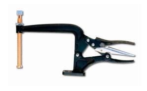
These locking pliers are specially made for welders. The thread is copper-plated so welding spatter will not stick to your pliers. The body is made of forged steel. When the copper-plated screw eventually shows wear, it can be replaced.
