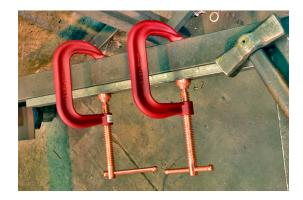
This handy G clamp is made of hardened and forged steel and is equipped with a spindle made of hardened C45 steel that is double copper-plated and protected against welding splashes. They have a large clamping force of 1800 kg and are available in different lengths.
