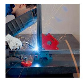
The Piher welding magnets can be used for welding 45 ° and 90 ° angles. They use a ferrite magnet protected with Bakelite resistant to high temperatures.
