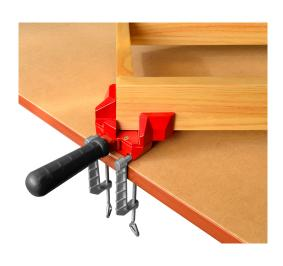
This table clamp with 8mm shaft can be used to fix products with an 8mm hole on your work table. Ideal for securing parallel clamps, corner clamps, etc. to ensure a stable clamping surface. Cast iron and aluminum body and steel thread. PE plastic protective cover included as standard.
