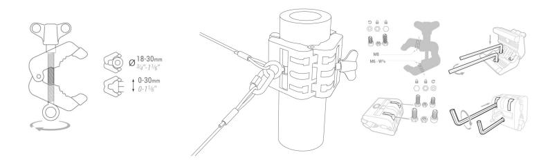
The Multiclamp is designed for use with the PIHER Multiprops telescopic supports, but can of course also be used separately.
