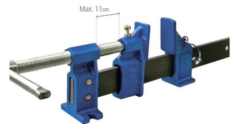
These extra sturdy panel clamps are ideal for climbing cabinet doors, frames, assembly panels, etc. Entirely made of steel and cast iron, making it indestructible. A solution for every job. Easily adjustable jaws. Extra resistant rolled steel bar (90KG / mm<sup>2</sup>), treated against rust and jaws coated with epoxy paint.
