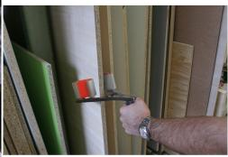
Panel carrier for easy lifting and moving of all types of sheet material. Full steel housing with rubber clamping brackets. This panel carrier can be used for wood, plastic, non-greasy metals and much more. Load capacity up to 75 kg.
