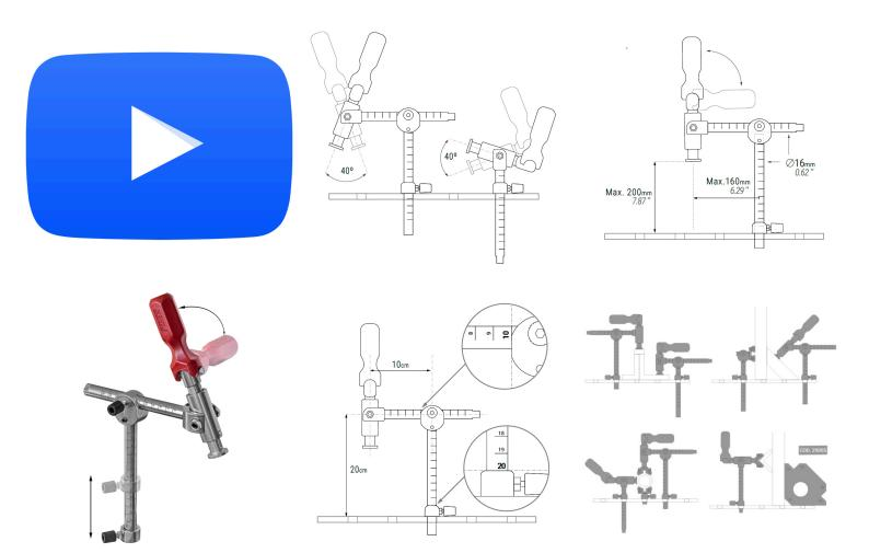
Designed with versatility to solve any clamping need on a welding table. Adaptable to any standard diameter. They feature an ergonomic PIHER handle with 3D joint position. Inside is a piston system with protected double fine screw thread. Horizontal and vertical clamping with a force of up to 350 kg. Adjustable up to 360 °. At the bottom there is a mobile stop that allows the shaft to be completely hidden under the table. The pressure surface has a mounting hole of M6 for mounting accessories.
