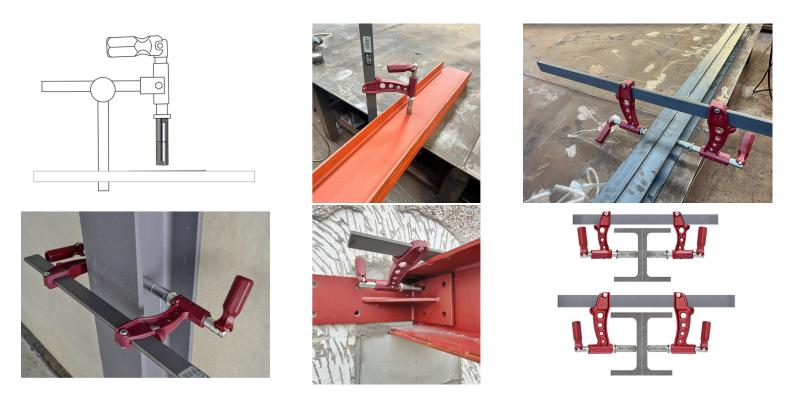
This piston extension is made of stainless steel and has a length of 4 cm. Assembly via M6 and M8 bolts. It can be easily mounted on the TCP clamp for welding tables and other clamps with an M6 or M8 mounting hole, increasing the clamping range.
