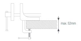
This portable carpenter vice can be easily mounted on all worktops with a thickness of up to 52mm. It is made of cast iron jaws and steel handle. The jaws have a width of 15cm, a height of 5.5cm and a maximum clamping thickness of up to 12cm.
