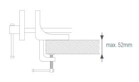
This portable carpenter vice can be easily mounted on all worktops with a thickness of up to 52mm. It is made of cast iron jaws and steel handle. The jaws have a width of 15cm, a height of 5.5cm and a maximum clamping thickness of up to 12cm.
