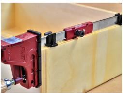
Accessory to connect two PRL400 parallel clamps together.
