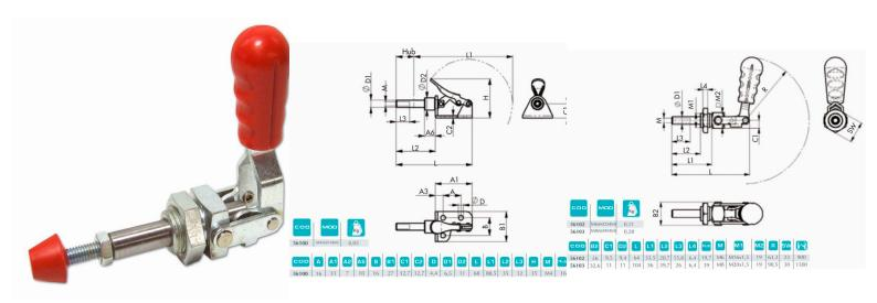
Push-pull quick clamps made of steel, with PVC handle and soft neoprene pressure foot to prevent damage to your workpiece. The clamps are available in different sizes and clamping force. All necessary dimensions can be found in the photos.
