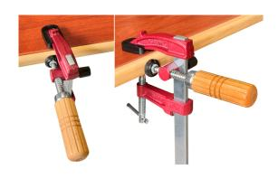
This single edge clamp can be used on all types of glue clamps with a maximum thickness of 8.5 mm. It is made from a steel body and has a galvanized thread. The handle is ergonomic and made of beech wood. Includes plastic protective cap. The edge clamp can be rotated out by a maximum of 50 mm and is therefore compatible with almost all types of screw clamps.
