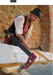
Sturdy spike fix for use on the PIHER Maxipress F clamps. Made from forged steel.
