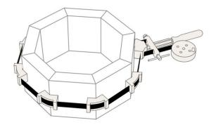
These steel band clamps from PIHER are super handy for assembly work. No more need for different clamps. They are equipped with an extra strong steel band (CK67S) with rounded corners, so the band cannot cut. The clamp itself is made of steel with a beechwood handle and nylon corners. Working with a steel band clamp ensures precise connections and evenly distributed pressure.
