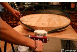
These steel band clamps from PIHER are super handy for assembly work. No more need for different clamps. They are equipped with an extra strong steel band (CK67S) with rounded corners, so the band cannot cut. The clamp itself is made of steel with a beechwood handle and nylon corners. Working with a steel band clamp ensures precise connections and evenly distributed pressure. Available in different sizes.
