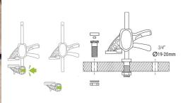
Using this accessory, you can easily use Piher's Mini Quick on workbenches with  $\emptyset$  19 mm or  $\emptyset$  20 mm holes. By removing one of the jaws of the Mini Quick, you can easily mount the rod in the accessory on the workbench, or mount the moving jaw horizontally. So this accessory can be used either horizontally or vertically, depending on your preference.
