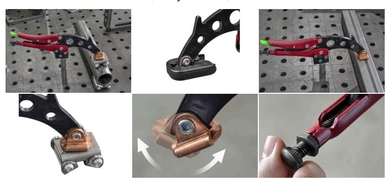
The TGA clamps, made of stainless steel, are available for Ø16 and 28 mm holes. Epoxy-coated handles, cataphoresis-coated pressure arm, and copper-plated swivel head prevent dirt from welding. Release with one click. M6 threaded hole for accessories. Rear screw controls power. Auto-Adjust technology always applies the
