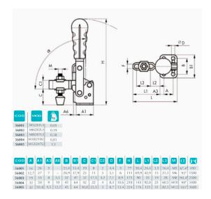
Vertical toggle clamps made of steel, with PVC handle and soft neoprene pressure foot to prevent damage to your workpiece. The toggle clamps are available in different sizes and clamping force. All necessary dimensions can be found in the photos.
