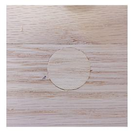
Plug cutters to be used on all wood types. These straight wood plug cutters are used to make plugs to be inserted after having drilled with "Forstner" bits. Use the plugs after installing sunken screws and sand the top of the plug flush with the wood surface to create nearly invisible screw connections on your wood projects. This cutter has a lenght of 140mm and 4 SP cutting teeth.
