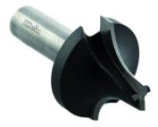
Quarter-circle concave radius cutter to easily and quickly round corners. The bit can also be used to create a flat-bottom groove between two quarter-round shapes. Increasing the working depth, you will obtain the classical "quarter-round" typical of dining table edges. Thanks to the high quality carbide cutting edges, this bit can be used efficiently on most types of wood.
