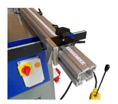
The Line Driller TT21EBM1 is a drilling machine for line boring with 1 drill chuck with 21 spindles and pneumatic operation.
