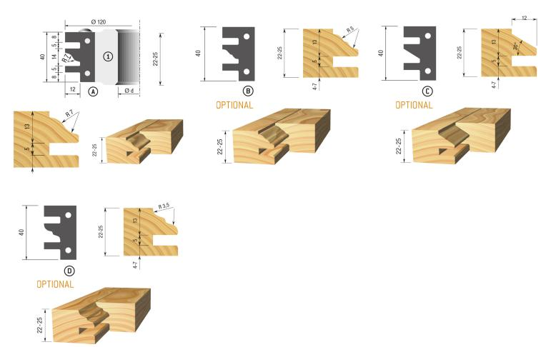
Cutter head in light metal with blades in high quality carbide (HW). Thanks to this cutter head you only have need of one tool to make joints with profile and counterprofile. Adjust the cutter head to the highest position to create the counterprofiles. Then lower the spindle back down to mill out the profiles. Suitable for use with wood of thickness 22-25mm. Thanks to the tungsten carbide blades, this cutter head cuts effortlessly through solid boards, solid woods or MDF.
