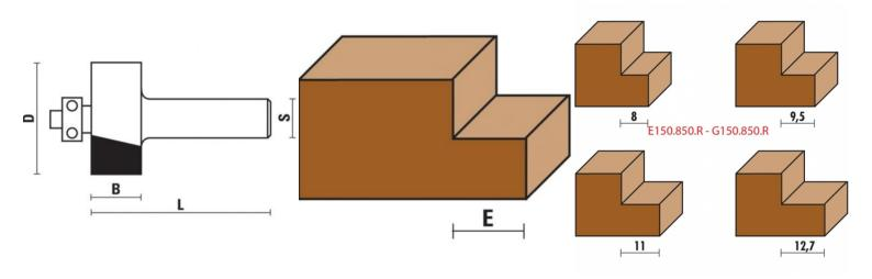
Used for making steps or rabbets on furniture, doors, tables and drawers. The bit is able to produce ultrasmooth cuts on both surfaces. These router bits are finished with carbide cutting edges. Thanks to these carbide cutting edges, the bit cuts effortlessly through most types of wood. You get the perfect result for all your projects and a long lifespan.
