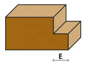
Used for making steps or rabbets on furniture, doors, tables and drawers. The bit is able to produce ultrasmooth cuts on both surfaces. These router bits are finished with carbide cutting edges. Thanks to these carbide cutting edges, the bit cuts effortlessly through most types of wood. You get the perfect result for all your projects and a long lifespan.
