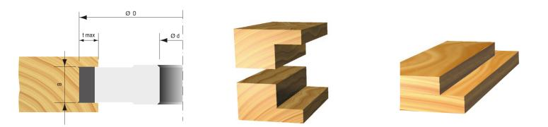
Cutterhead with alternate shear reversible knives and spurs in high quality carbide (HW). The blades have an
